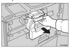
4 Lift upper drum stay B3 a little to unlock the drum unit, then pull
