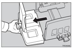
2 Adjust the end plate to match the paper size scale on the opposite side of the operation panel.
