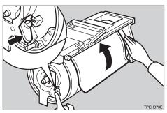
With a dry soft cloth, remove any ink that has accumulated on the trailing edge of the drum unit.
