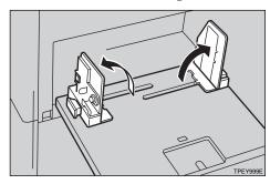
Grasp the side/end plate knob and adjust the side/end plates to match the paper size.
