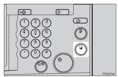
After the first set is completed, set the second original on the exposure glass (contact glass) and press the [Start] key.
