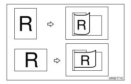
When you have an optional memory board and the original is set in a different direction from the print paper, the machine automatically rotates the original image by 90° to match the print paper direction.
