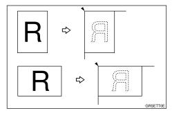
When you have an optional memory board and the original is set in a different direction from the print paper, the machine automatically rotates the original image by 90° to match the print paper direction.
