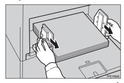
To print on thin paper  $(47.1 \text{ g/m}^2, 12.5 \text{ lb})$ , slide the levers (behind the paper feed side/end plates) in the direction of the arrow (see illustration).
