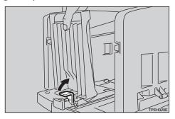
Adjust the end plate angle by turning the screw clockwise or counterclockwise.
