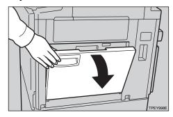
2 Lift the feed side/end plates.
