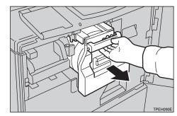
Lift upper drum stay B3 a little to unlock the drum unit, then pull
