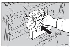
**8** Lift the drum unit lock lever.
