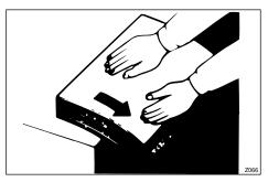
• When paper edges stick together or paper is not fed to the machine, shuffle the paper as shown.
