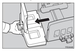
Adjust the end plate to match the paper size scale on the op-
