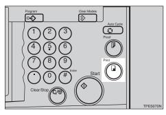
After the first set is completed, set the second original on the exposure glass (contact glass) and press the [Start] key.
