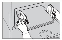
To print on thin paper (47.1 g/m<sup>2</sup>, 12.5 lb), slide the levers (behind the paper feed side/end plates) in the direction of the arrow (see illustration).
