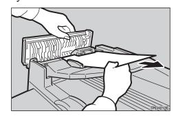
If you cannot remove misfed original in step **2**, open the document feeder. Pull the green knob towards you and remove the misfed original.
