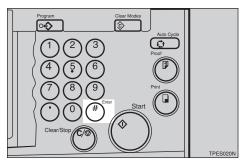
Adjust the vertical page numbering position with the Number keys.
