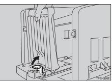
**2** Adjust the end plate angle by turning the screw clockwise or counterclockwise.
