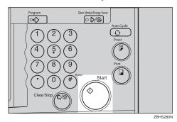
Use the 【◀】 or 【▶】 key to adjust the printing speed. The relationship between printing speed and print quality depends on the type of paper you use.
