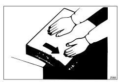
When paper edges stick together or paper is not fed in, shuffle the paper as shown.
