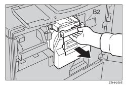
Lift upper drum stay B3 a little to unlock the drum unit, then pull out the drum unit while holding drum unit handle B2 and upper drum stay B3.
