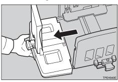
2 Adjust the end plate to match the paper size scale on the opposite side of the operation panel.
