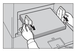
To print on thin paper (47.1g/m<sup>2</sup>, 12.5 lb), slide the levers behind the paper feed side plates in the direction of the arrow (see illustration).
