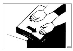
When the leading edge margin of the original is less than 10mm, 0.4" or there is a solid image on the leading edge, insert the original with the widest margin first or make a leading edge margin by making a copy.
