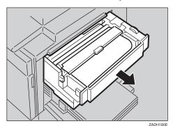
2 Open the black cover at the bottom of the master tray and remove turn scraps of the master.
