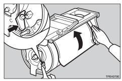
Insert the drum unit until it locks in position, then lower the drum unit lock lever.
