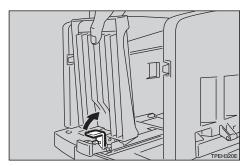
2 Adjust the end plate angle by turning the screw clockwise or counterclockwise.
