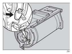
Insert the color drum unit along the guide rail.
