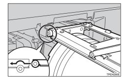
**2** Lower drum unit lock lever B1 of the inserted drum.
