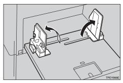
**3** Grasp the side/end plate knob and adjust the side/end plates to match the paper size.
