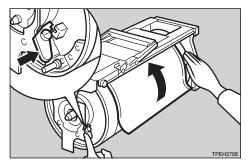
**1** Insert the drum unit until it locks in position, then lower the drum unit lock lever.
