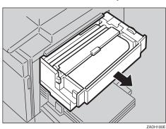
**2** Open the black cover at the bottom of the master tray and remove turn scraps of the master.
