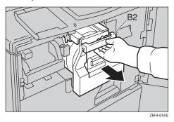
Lift upper drum stay B3 a little to unlock the drum unit, then pull out the drum unit while holding drum unit handle B2 and upper drum stay B3.
