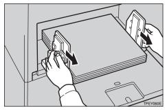
To print on thin paper  $(47.1g/m^2, 12.5 \text{ lb})$ , slide the levers behind the paper feed side plates in the direction of the arrow (see illustration).
