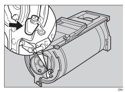
**1** Insert the colour drum unit along the guide rail.
