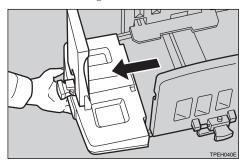
Adjust the end plate to match the paper size scale on the opposite side of the operation panel.
