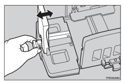
**2** Grasp the side plate knobs and move the paper delivery side plates to match the print paper size.
