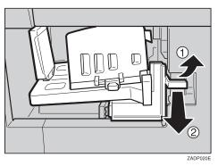
**2** Pull the front paper delivery side plate down towards you to open it, then remove the prints.
