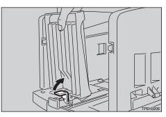
2 Adjust the end plate angle by turning the screw clockwise or counterclockwise.
