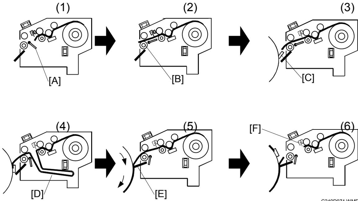
The duct plate [A] is in the middle position before printing. (1)
