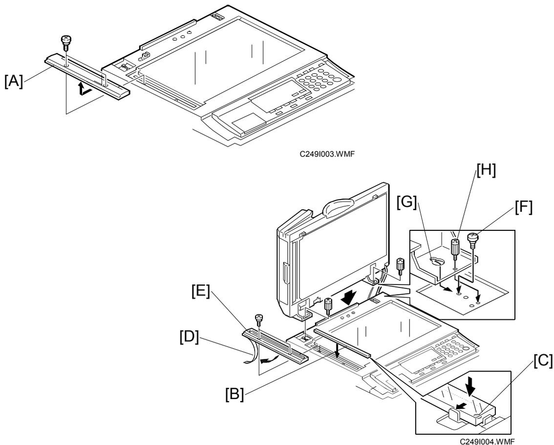
2. Remove the left scale [A] (2 screws).
