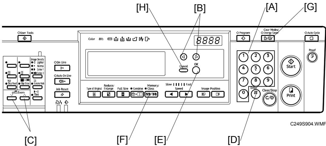
1. Using the number keys [A] or the <> keys [B] or the zoom keys [C], enter the desired main menu number (listed below), then press the Enter key [D] or the OK key [E].
