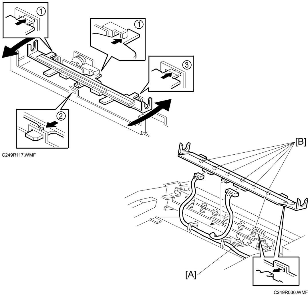
1. Insert in the nails (①) to the operation side and middle.
