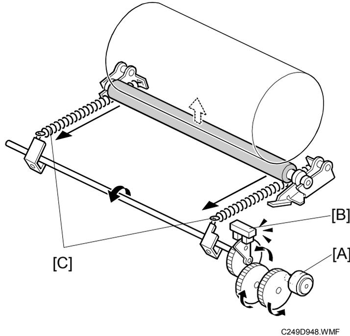
The printing pressure motor [A], the printing pressure sensor [B] and printing pressure spring [C] were added to the press roller to control the image density of each printing speed or temperature. The printing pressure depends on temperature and printing speed, as shown in the following table.
