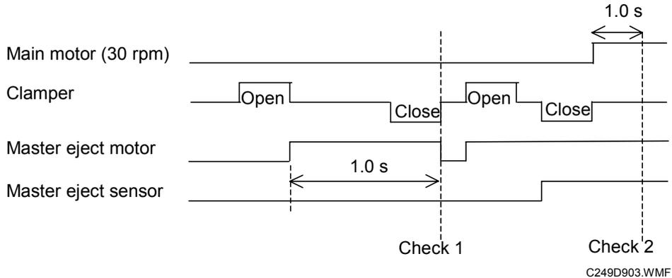
**Jam check timing:** When the clamper open sensor is on (clamper open).
