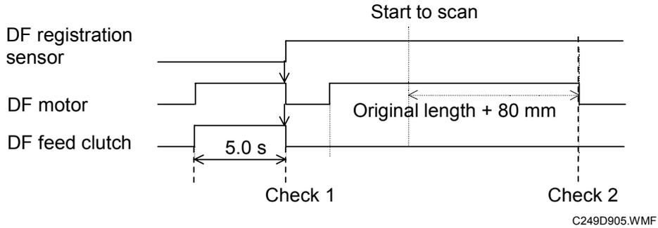
**Jam check timing:** When an original is placed in the DF.
