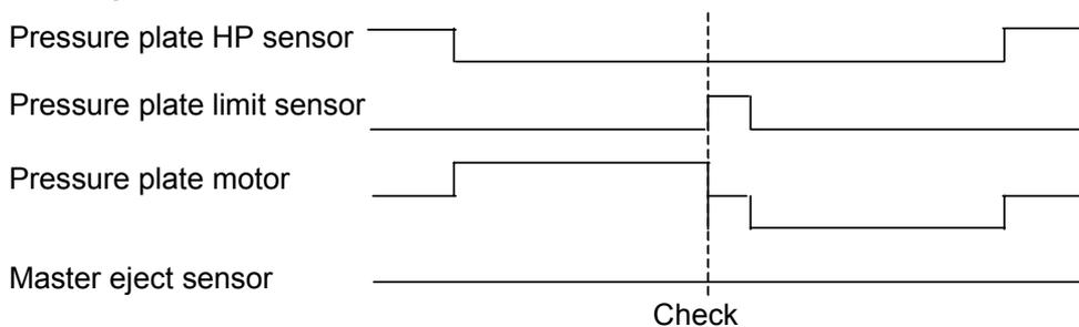
**Jam check timing:** When moving the pressure plate.
