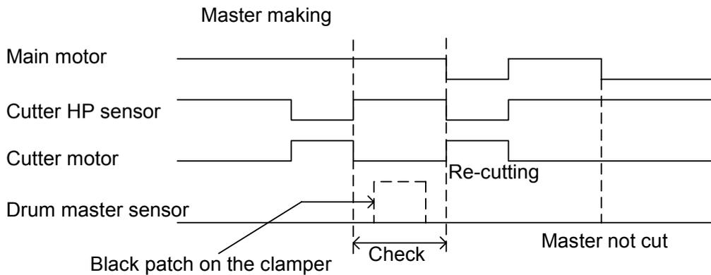
**Jam check timing:** When the master is clamped in the clamper and cutting is taking place.
