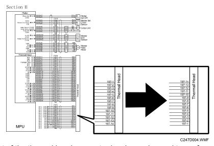
The pin layout of the thermal head connector has been changed to conform to the new thermal head.
