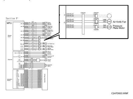
The air knife fan motor previously connected to CN347 has been deleted (no. of motors reduced from 2 to 1).
