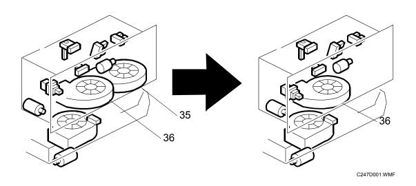
The number of air knife fan motors has been decreased from 2 to 1, due to the decrease in size of the printable image area.
