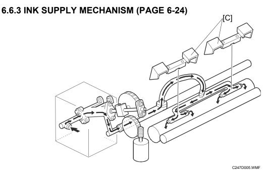
Two ink pipe covers [C] have been added to ensure that ink from the ink distributor does not stick to the ink sensor.
