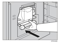
**8** Lower the drum unit lock lever.
