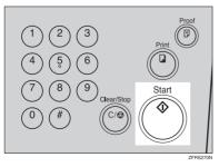
Printing starts automatically after trial print is delivered.
