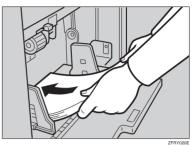
4 Make sure that the paper feed side plates touch the paper lightly. Shift the lock lever backward.
