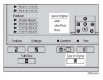
**2** Press the [Image Density] key to adjust the image density.
