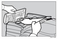
**3** If you cannot remove the misfed original in step **2**, lift the document feeder.
