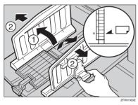
**E** Lift the paper delivery end plate and move it to match the print paper size.
