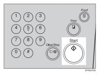
Printing starts automatically after trial print is delivered.
