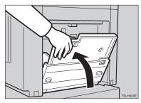
4 Move the end plate until the plate handle is flush with the end of the tray.
