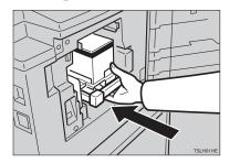
**8** Lower the drum unit lock lever.
