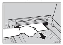
**1** If you still cannot remove the misfed paper, press the ADF open lever and open the ADF unit to remove the original.
