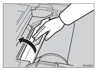
4 Remove the used master roll and pull out both spools. Then, insert both spools into a new master roll.
