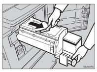
**5** Remove the drum unit from the machine while holding the upper drum stay.
