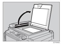
2 Set the original face down on the exposure glass. The original should be centered according to the size marks on the right scale.
