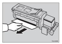
**B** Remove paper that is stuck to the drum.
