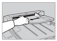
**2** Insert the aligned originals face up in the document feeder until they stop.
