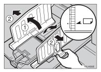
**B** Lift the paper delivery end plate and move it to match the print paper size.
