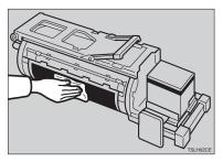
**5** Insert the drum unit until it locks in position, then lower the drum unit lock lever.
