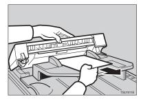
**1** If you cannot remove the misfed original, pull out the original from the side of the original tray and remove the original.
