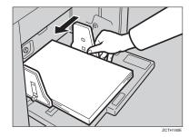
**B** When you finish prints, position pressure lever to the Standard paper position.
