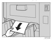
**2** If the paper is completely wrapped around the drum, pull out the drum unit and remove the misfed paper from the drum.
