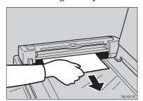
4 If you still cannot remove the misfed paper, press the ADF open lever and open the ADF unit to remove the original.
