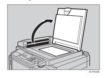
2 Set the original face down on the exposure glass. The original should be centred according to the size marks on the right scale.
