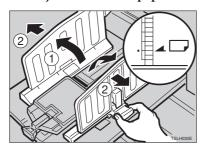
Lift the paper delivery end plate and move it to match the print paper size.
