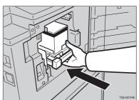
**8** Lower the drum unit lock lever.
