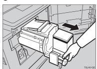
• Lift the lever to unlock the drum unit and pull out the unit.
