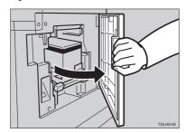
**2** Pull out the ink holder and remove the used ink cartridge.
