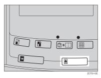
Press the [Image Density] key to adjust the image density.
