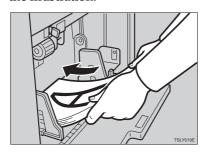
**12** Exchange the drum unit. See ⇒ P.52 "Changing the colour Drum Unit".
