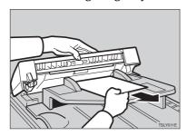
3 If you cannot remove the misfed original, pull out the original from the side of the original tray and remove the original.
