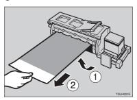
**4** Re-insert the drum unit until the drum unit locks in position and put the lever back in place.
