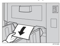
2 If the paper is completely wrapped around the drum, pull out the drum unit and remove the misfed paper from the drum.
