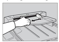
2 Insert the aligned originals face up in the document feeder until they stop.
