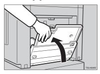
Move the end plate until the plate handle is flush with the end of the table.
