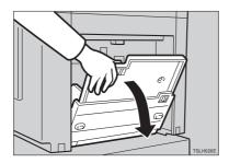
Put the paper feed side plates lock lever. Adjust the side plates to match the paper size.
