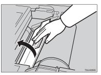
4 Remove the used master roll and pull out both spools. Then, insert both spools into a new master roll.
