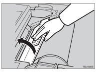
4 If you could not remove the misfed master in steps 2 and 3, take out the drum and remove the misfed master from the inside.
