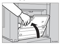
4 Move the end plate until the plate handle is flush with the end of the table.
