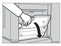
**2** Put the paper feed side plates lock lever. Adjust the side plates to match the paper size.
