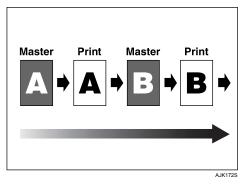
Master making and printing are completed continuously.
