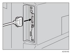
**2** Attach the other end of the parallel interface cable to the port of the computer. Secure the interface cable.
