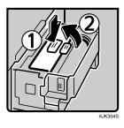
**B** Rotate the spool backward to remove the remaining masters.
