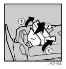
If you cannot remove the misfed original, open the ARDF external cover, and then remove the misfed original.
