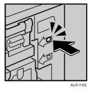
**3** Lower drum unit lock lever (B1).
