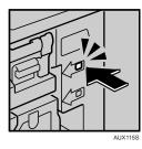
**3** Lower drum unit lock lever (B1).
