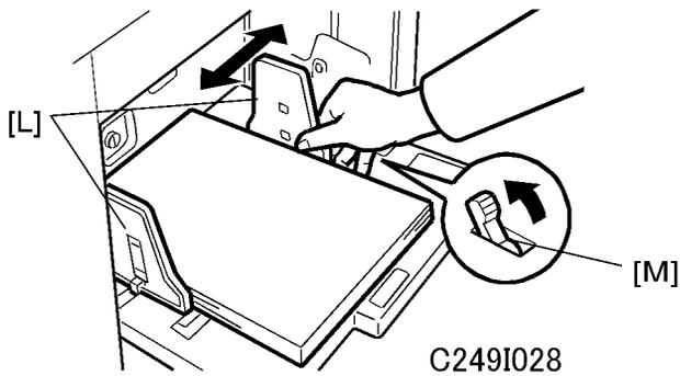
12. Open the paper table, and load a stack of paper.
