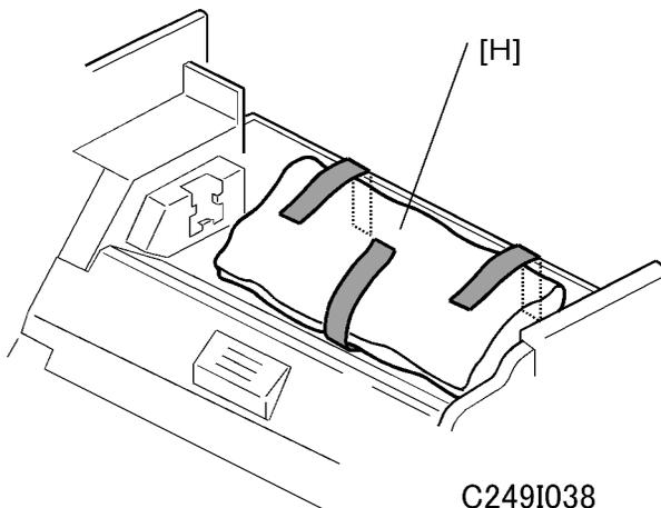
5. Pull out the master making unit, and take out the accessory bag [H].
