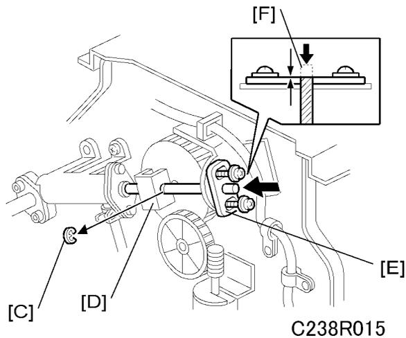
1. Remove the E-ring [C] to free the plunger from the pump drive slider [D].
