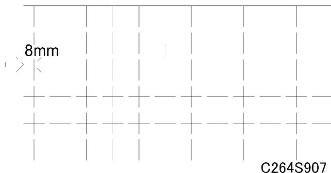
6. If this distance is not 8 mm, access SP6-101 to 107 and then input a value to adjust the distance (range: -40 to 40, step: 1) for each of 6 copy samples.
