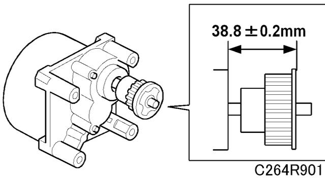
After putting the pulley back on the main motor shaft, refer to the above illustration for the correct position of the pulley.
