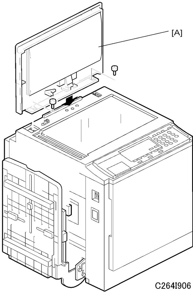
1. Install the platen cover [A] (2 screws).
