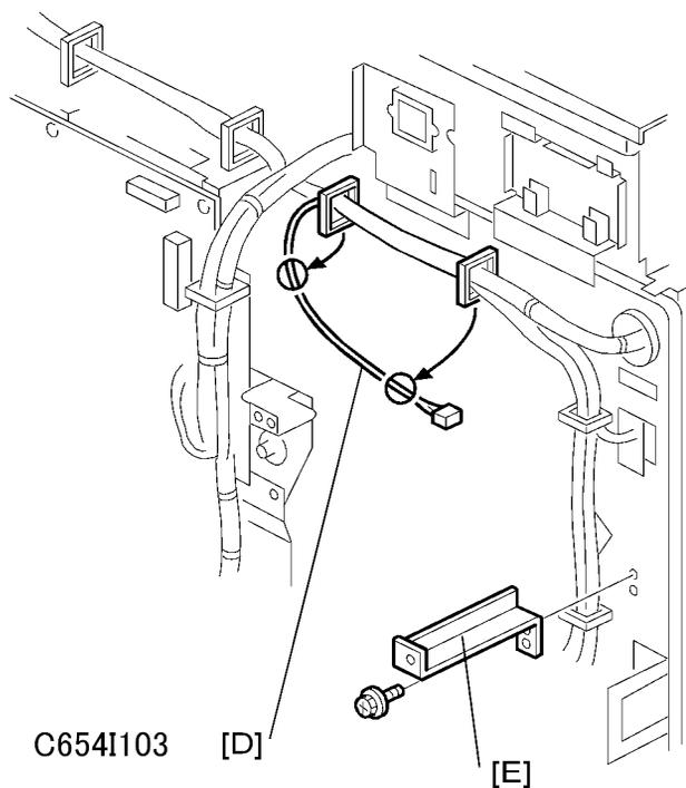
3. Open the two clamps to release this part of the harness [D], which will be connected to the controller.
