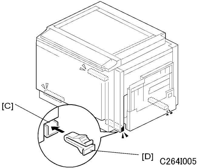
2. Push the carrying handles [C] into the machine, and attach the carrying handle stoppers [D].
