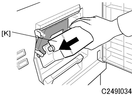
11. Open the door, and insert a new ink cartridge [K].
