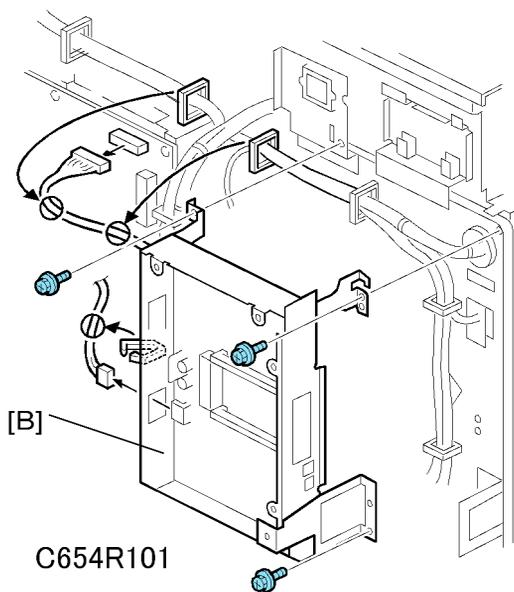
2. Remove the printer board with case [B] (⚙️ x 3, 📡 x 2, 🖨️ x 3).
