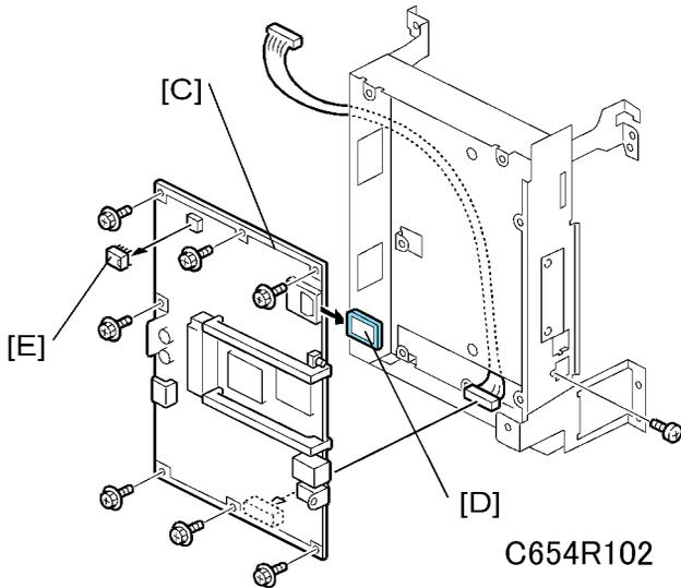
3. Remove the printer board [C] from the case (⚙️ x 8, 📡 x 1).
