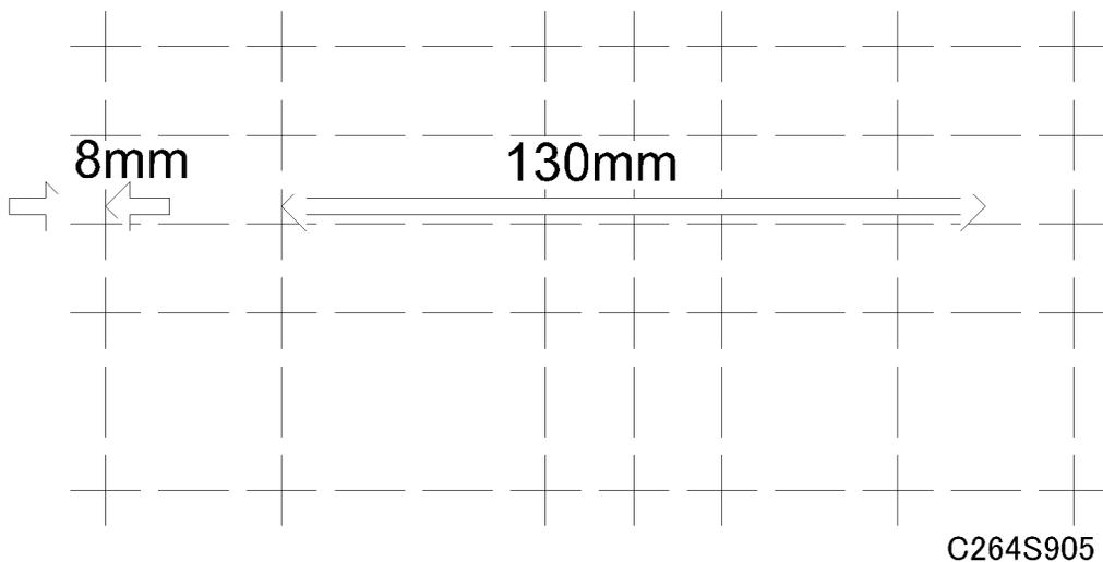
1. Input SP8-10 (Test patterns) and enter "6", then press the Start key.
