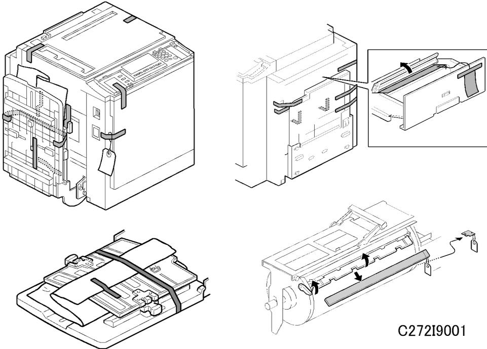
3. Remove the filament tape and string securing the covers and units as shown above.
