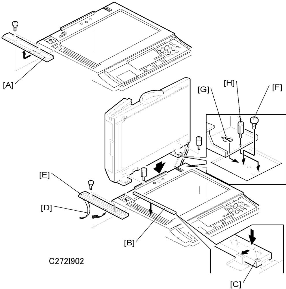
2. Remove the left scale [A] (2 screws).
