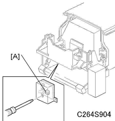
Access SP6-40, and open the door cover. Then turn VR1 [A] on the ink detection board until the display becomes "3.0 u" (3 us).
