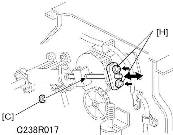
7. Re-tighten the two screws [H].
