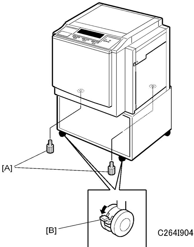
1. Unpack the box. When installing the optional table, mount the machine as shown (there are 2 screws [A] packed with the table).
