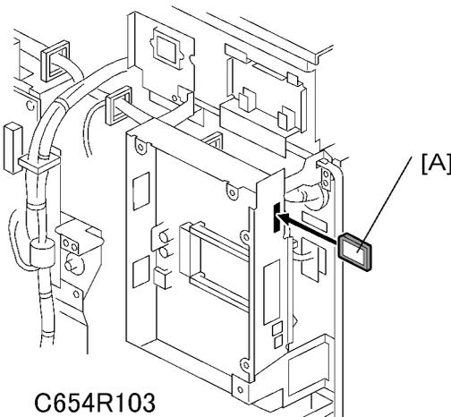
3. Put the SD card [A] in the slot of the ACU board.
