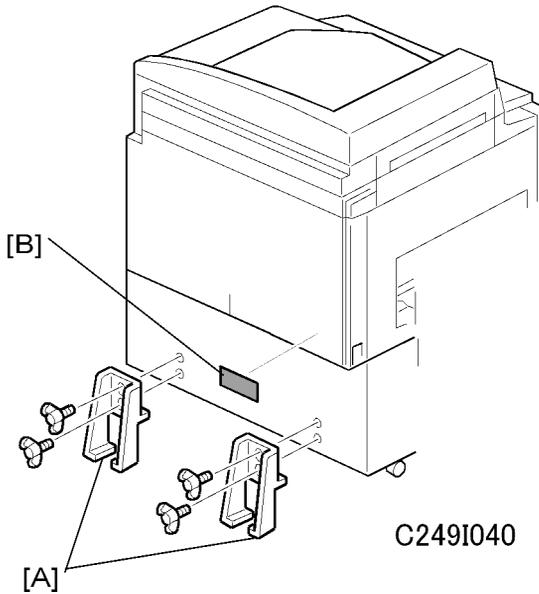
1. Attach the two stabilizer brackets [A] to the back of the table using the thumbscrews (4 screws).
