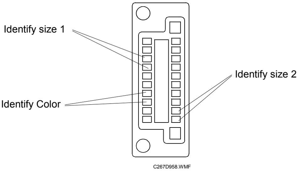
The type of drum is distinguished by inserting jumper wires in the drum connector [A] at three locations, as shown in the lower diagram.
