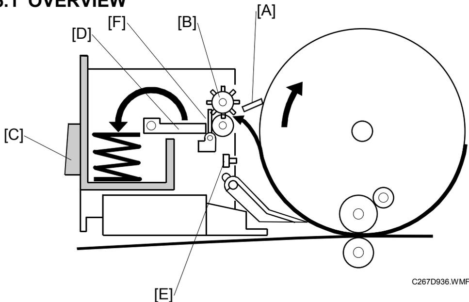
The master eject unit removes the used master from the drum. (🖨️📄: Digital Duplicators – Duplicating Process – Master Ejecting)
