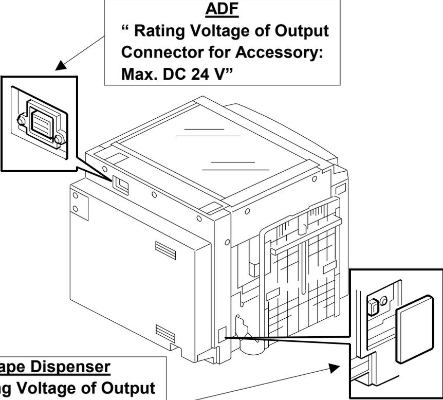
The diagram shows a perspective view of a device with two callout boxes. The top callout box points to a power socket on the top surface of the device. The bottom callout box points to a power socket on the front panel of the device. Both callout boxes contain text regarding the maximum DC voltage rating for accessories connected to those sockets.
