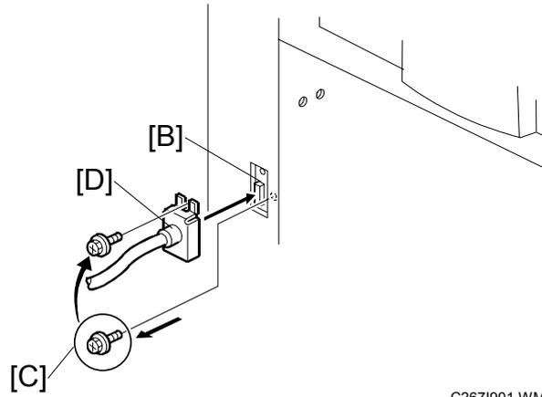
4. Connect the harness from the tape dispenser to the connector [B].
