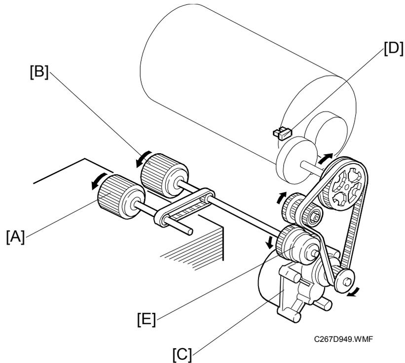
The pick-up roller [A] and paper feed roller [B] are driven by the main motor [C] through gears and a timing belt.
