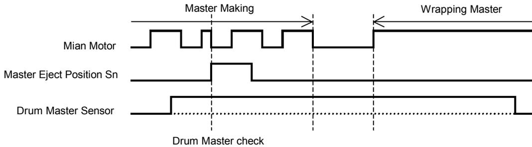
A master clamp error occurs when the drum master sensor does not turn on at the home position (the drum stops at the home position for a short time; home position is when the master eject position sensor turns on).
