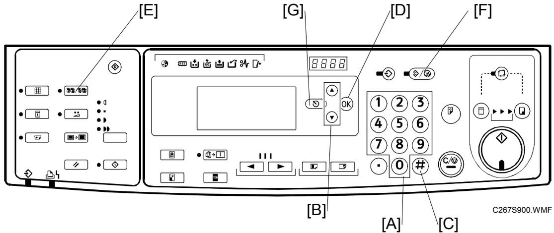
1. Using the number keys [A] or the  $\Delta \nabla$  keys [B], enter the desired main menu number, then press the Enter key [C] or the OK key [D].
