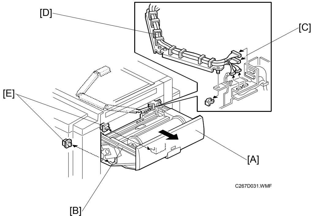
The master making unit [A] can be pulled out along the guide rails [B].
