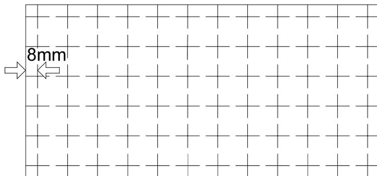
4. If this distance is not 8mm, access SP6-101 to 104 and then input a value to adjust the distance (range: -40 to 40, step: 1) for each of 3 copies samples (i.e. 30, 60, 80, 100 and 130 rpm samples). The higher the value, the narrower the distance between the leading edge and 1st line becomes (and vice-versa). Also, each step corresponds to approximately 0.5mm. Input the value that will bring the distance to 8mm.
