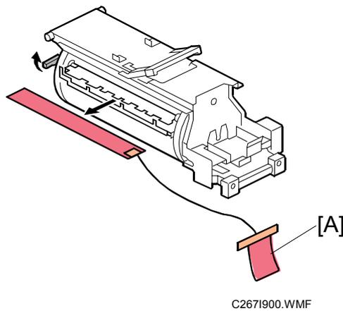
1. Remove the protective sheets [A] from the drum.
