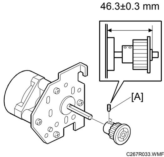
**NOTE:** Tight the screws alternately little by little. Do not tighten them completely one by one.
