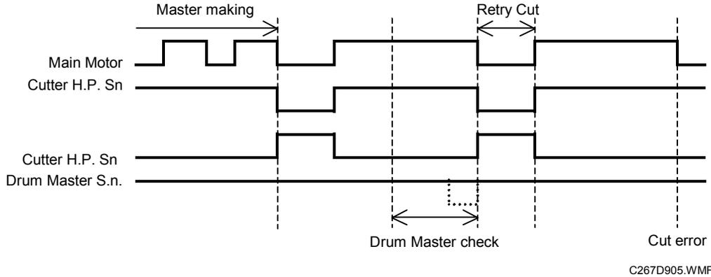
The drum master sensor does not turn on between feed start timing sensor and drum black patch after the master cutting operation. In this case, the machine tries to cut the master again and if the machine does not cut the master correctly, the D jam indicator lights.
