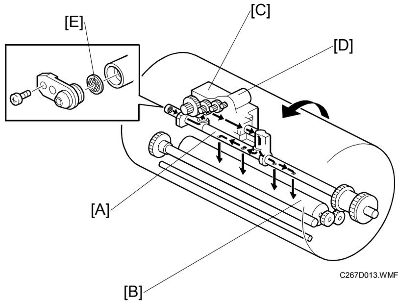
Ink is supplied from the ink cartridge to the ink roller [B] by a trochoid type pump [C]. The ink pump is driven by the ink supply motor (a dc motor) [D].
