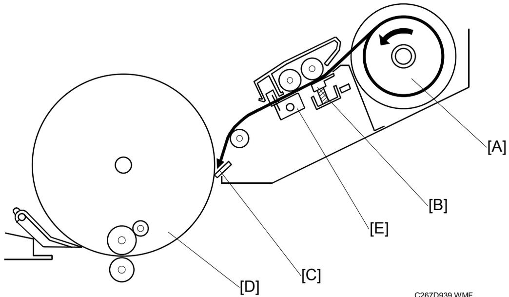
The master making unit makes an image on the master and feeds the master to the drum. (☛☛: Digital Duplicators – Duplicating Process – Master Feeding)
