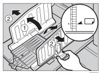
Lift the paper delivery end plate and move it to match the print paper size.
