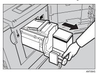
2 Unlock the lever to open the clamp of drum unit.
