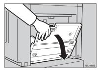
2 Shift the paper feed side plates lock lever forward. Adjust the side plates to match the paper size.
