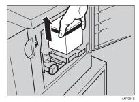
Remove the cap of the new ink cartridge.
