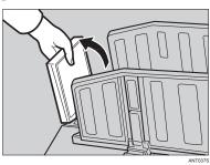
Lift the paper delivery end plate and adjust it to match the paper size.
