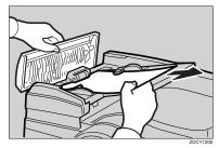
If you are unable to remove the misfed original in Step **2**, lift the Auto Document Feeder.
