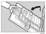
2 Lift the paper delivery side plates and adjust them to the paper size.
