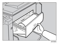
2 Open the master feeding cover, and then remove the misfed master inside.
