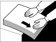
If you are unable to correct the paper curl, place the paper in the paper feed tray with it curling either upward or downward, as shown in the illustration below.
