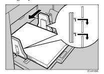
A Shift the lock lever to its original position.
