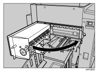
**5** If the indicators remain lit, open the front cover and close it firmly or press [OK] key.
