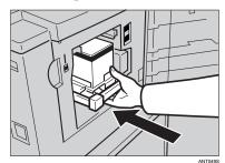
**1** Lower the drum unit lock lever.
