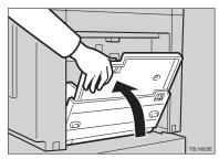
Move the end plate until the plate handle is flush with the end of the tray.
