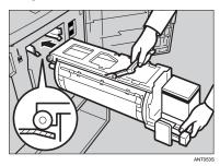
Slide in the drum unit until it locks into position.
