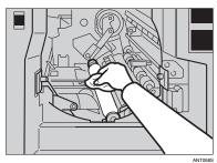
**5** Insert the drum unit until it locks into position, and then lower the drum unit lock lever.
