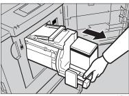
For details about how to remove the drum unit, see p.120 "Maintaining the Machine".
