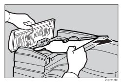
If you are unable to remove the misfed original in Step **2**, lift the Auto Document Feeder.
