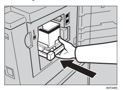
**1** Lower the drum unit lock lever.
