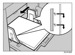
**A** Shift the lock lever to its original position.
