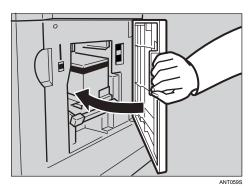
Either a master misfeed has occurred either in the master eject section, or the master is wrapped around the drum unit.
