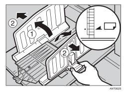
2 Lift the paper delivery end plate and move it to match the print paper size.
