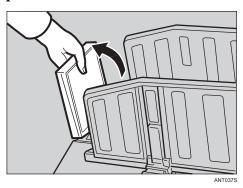
4 Lift the paper delivery end plate and adjust it to match the paper size.
