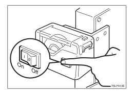
Press the manual cut button to trim off the leading edge of the tape.
