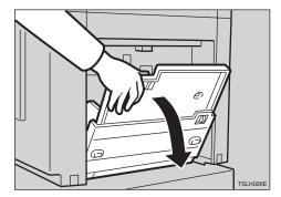
2 Shift the paper feed side plates lock lever forward. Adjust the side plates to match the paper size.
