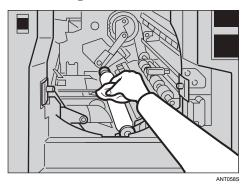
**5** Insert the drum unit until it locks in position, and then lower the drum unit lock lever.
