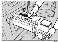
Remove the drum unit from the machine while holding the upper drum stay.
