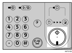
6 After the first original has been scanned, place the second original in the same way.
