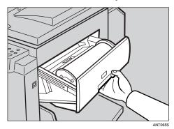
Press the release button to open the master feeding cover.
