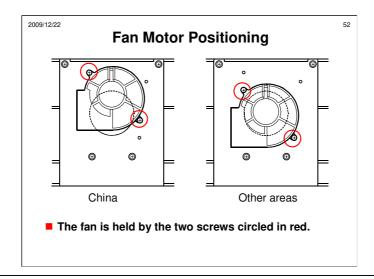
In the upper position (China), the fan does not pull the paper against the transport belts so strongly.
