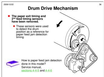
The only difference is the removal of these two sensors. Jam detection is done by counting main motor encoder pulses, as in the Silver, and this can be done without the two sensors.
