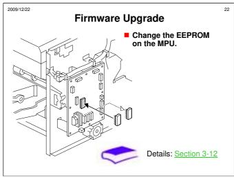
To change the firmware, change the EEPROM on the MPU board. Now, take a look at the procedure in the service manual (section 3-12).
