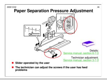
If the user has non-feed or multi-feed problems, they can adjust the lever position (the default position is 3).
