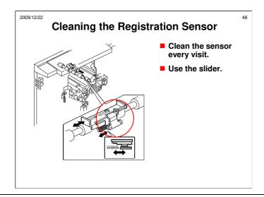
Some types of paper generate a lot of dust, which can lead to registration sensor errors.
