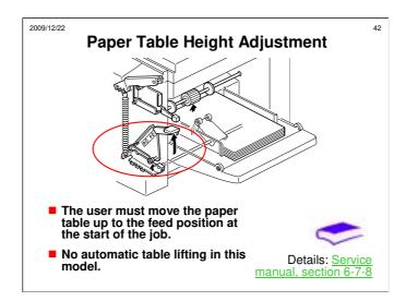
Note the two levers on the left side of the feed table.
