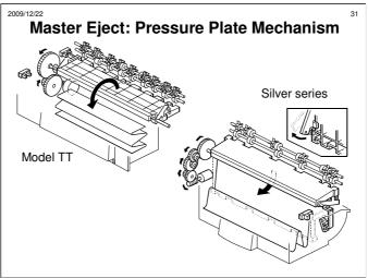
Here is another pair of diagrams to compare the mechanisms in the new and old models.
