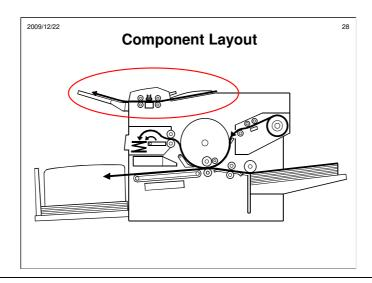
The only large component that is completely different from the Silver series is the scanner (circled in red).
