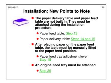
This slide covers the main differences between installation for this machine and for models in the Silver, Silver-V, and Silver-V2 series.
