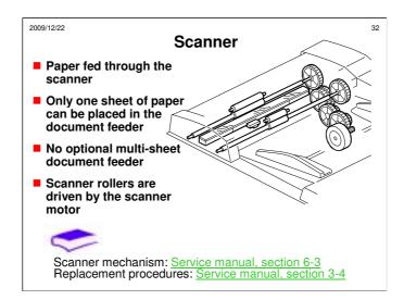
This shows the scanner mechanism.
