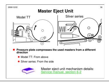
The mechanism is very similar to the Silver, except for the point noted above. For details of all mechanisms in the master eject unit, click on the link at the bottom of the slide.
