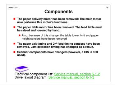
This machine is a simplified version of the Silver series, and some of the components have been removed. Details are listed above.
