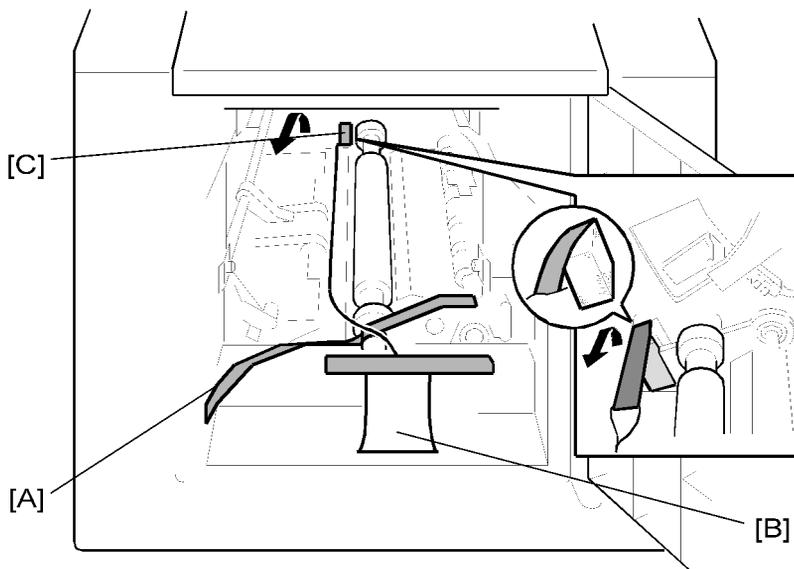
3. Remove the front tape [A], the tag [B], and the rear tape [C].
