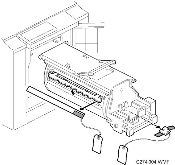
1. Unpack the machine and remove all the wrapping.
