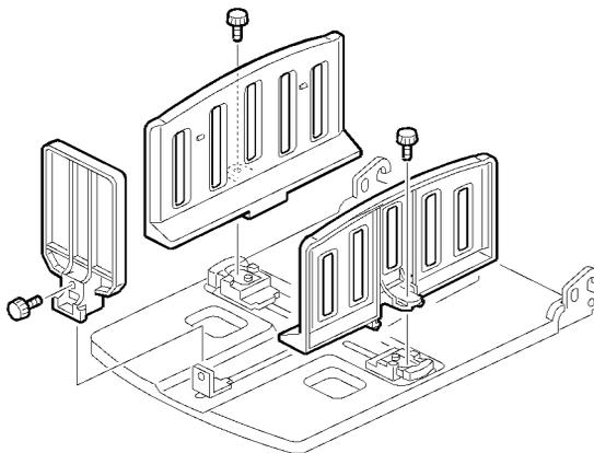
15. Attach the side and end fences, as shown. (⚙️ x 3)
