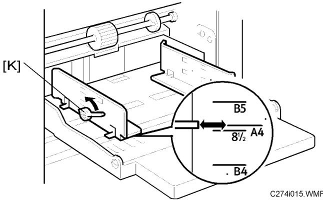
17. Release the paper feed side plate lock levers [K] and adjust the side plates to match the paper size.
