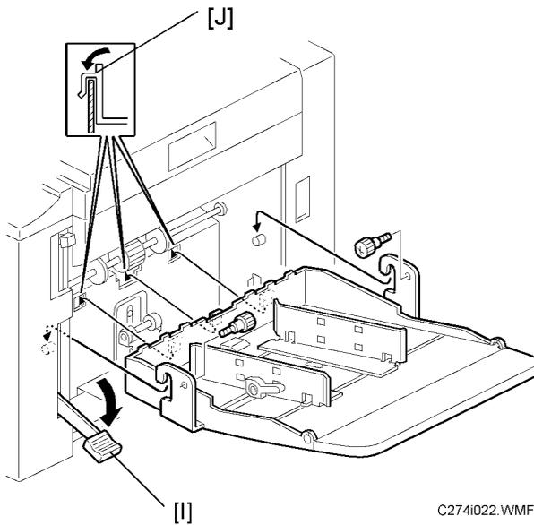
14. Lower the paper feed tray adjustment lever [I], and install the paper table. (⚙️ x 2)
