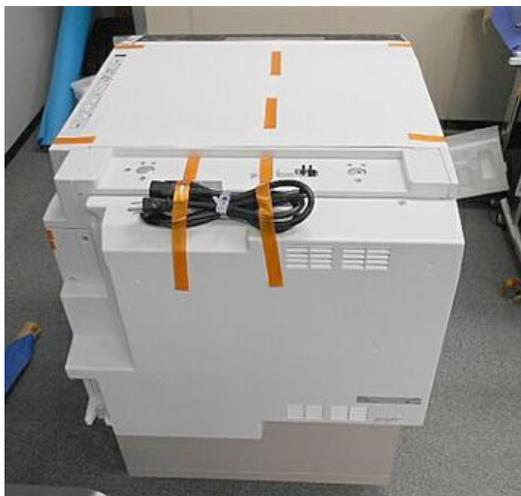
4. Remove the tape, shipping materials, and the power cord from outside the machine.
