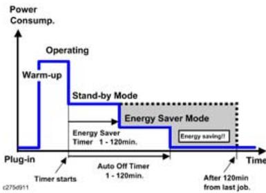
The area shaded grey in this diagram represents the amount of energy that is saved when the timers are at the default settings. If the timers are changed, then the energy saved will be different. For example, if the timers are all set to 120 min., the grey area will disappear, and no energy is saved before 120 min. expires.
