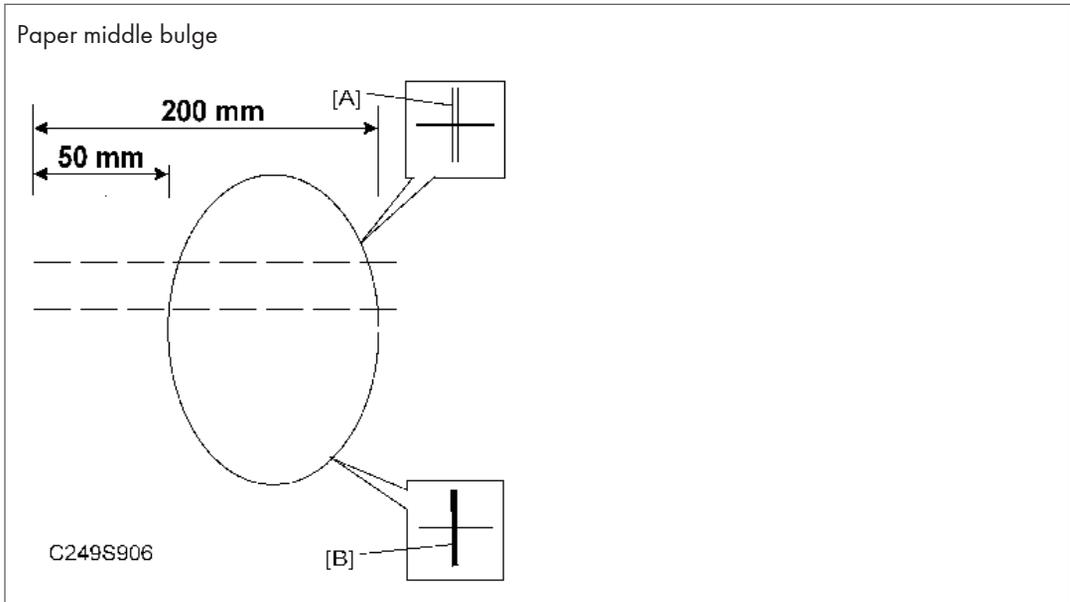
Adjusts doubled [A] or blurred [B] images (e.g. bold lines, text) for each printing speed (15, 30, 60, 75, 90, 105, 130 rpm), by changing SP settings.
