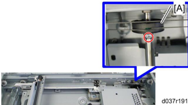
10. Rear scanner drive pulley [A] (🔩 × 1)
