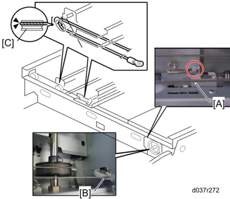
6. Hook the right end onto the front scanner wire bracket [A]. The end should go via the rear track of the right pulley [B] and the rear track of the movable pulley [C].
