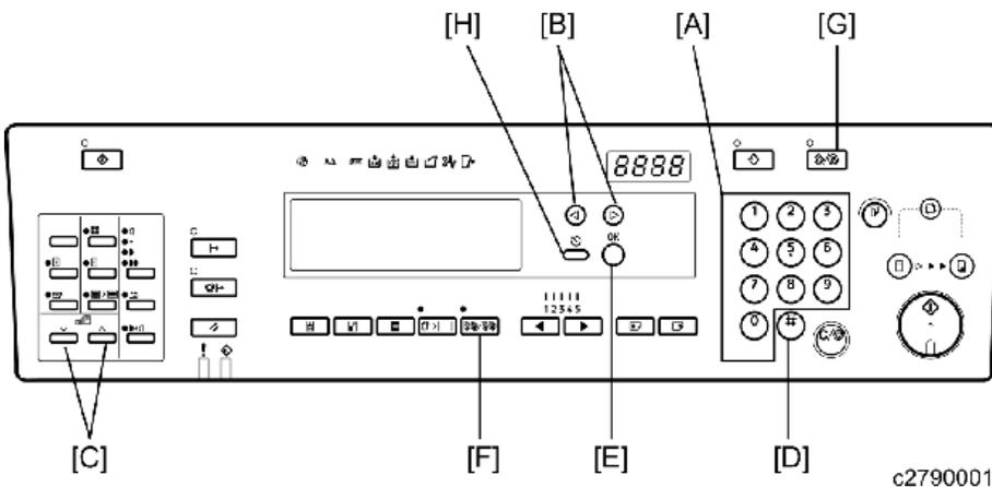
1. Using the number keys [A] or the <math>\triangleleft</math> keys [B] or the zoom keys [C], enter the desired main menu number (listed below), then press the Enter key [D] or the OK key [E].
