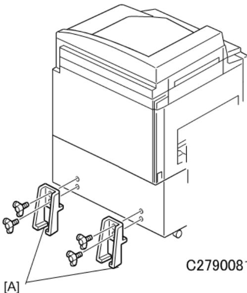
1. Attach the two stabilizer brackets [A] to the back of the table using the thumbscrews (🔩 x 4).
