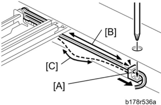
Run the cable so there is no slack. Slide the adjustor clamp [A] to adjust the cable slack.
