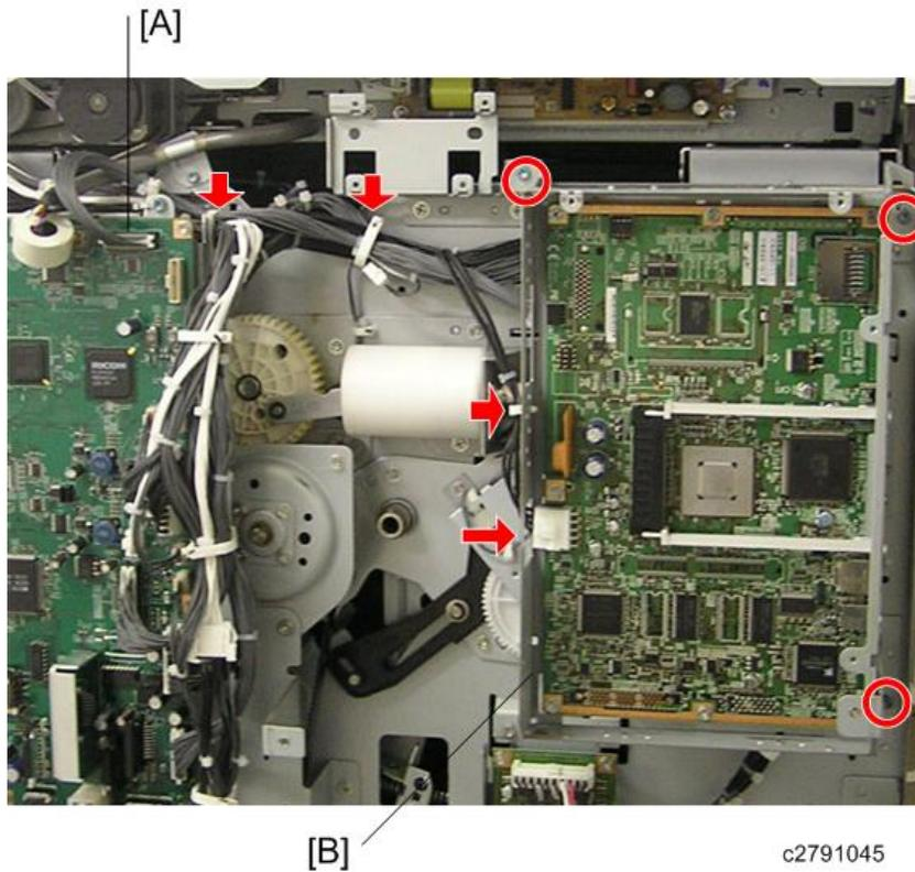
2. Remove the printer board with case. (🔧 × 3, 🛠 × 2, 🛠 × 3).
