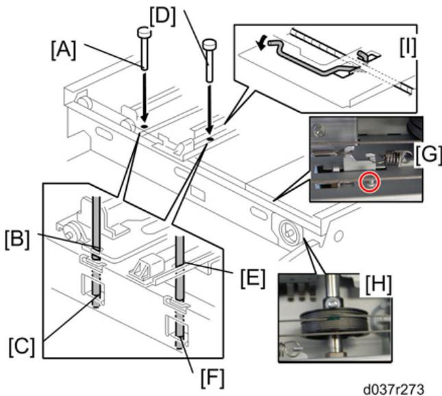
8. Insert a scanner positioning pin [A] through the 2nd carriage hole [B] and the left holes [C] in the front rail. Insert another scanner positioning pin [D] through the 1st carriage hole [E] and the right holes in the front rail [F].
