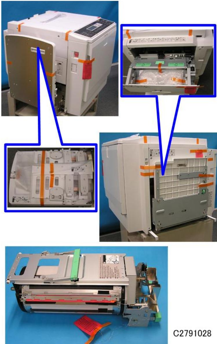
3. Remove the filament tape and string securing the covers and units as shown above.
