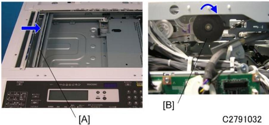
3. Move the 1st scanner carriage [A] to the right side by rotating the scanner motor [B] clockwise.
