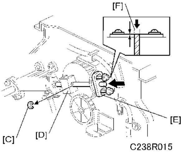
1. Remove the E-ring [C] to free the plunger from the pump drive slider [D].
