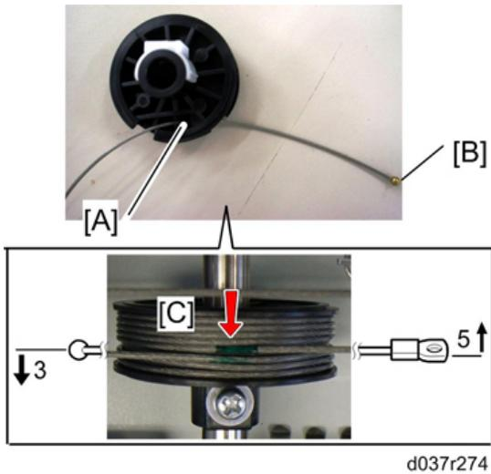
1. Position the center ball [A] in the middle of the forked holder.
