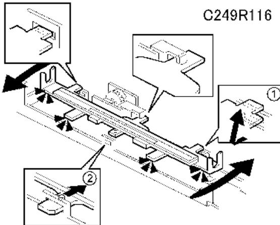
6. Turn the thermal head clockwise and remove a tab (1).
