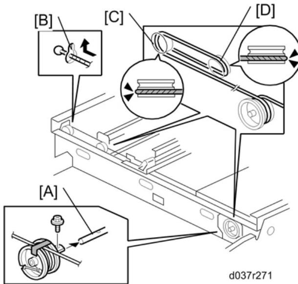
4. Install the drive pulley on the shaft [A] (⌀ × 1, ⌀ × 1).
