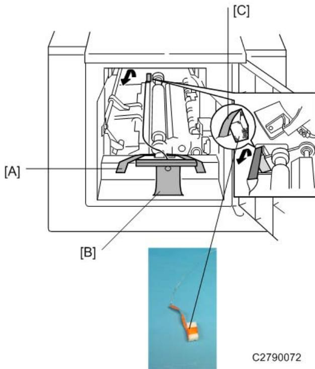
4. Remove the front tape [A], the tag [B], and the rear tape [C].
