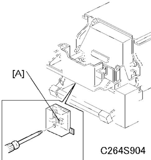
Access SP6-40, and open the door cover. Then turn VR1 on the ink detection board until the display becomes "3.0 u" (3 us).
