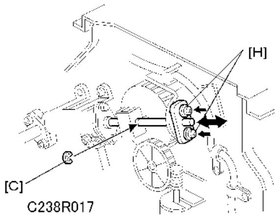
7. Re-tighten the two screws [H].
