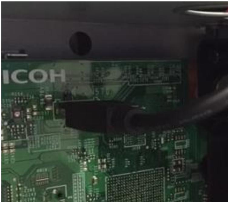
**Figure 8: USB connector (IPU)**
