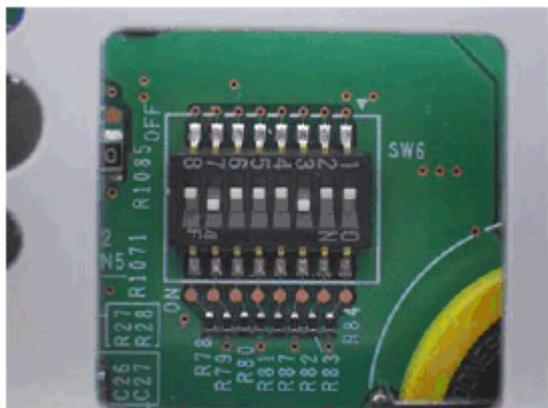
The DIP switch No.1 turns ON/OFF the SC reduction function. Change the setting when needed.
