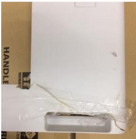
Figure.4 Broken right rear cover
