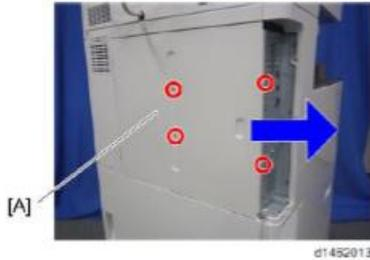
6. Remove the scanner rear cover [A] (screws x 3)
