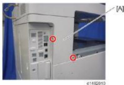
4. Remove the controller cover [A] (screws x 4)
