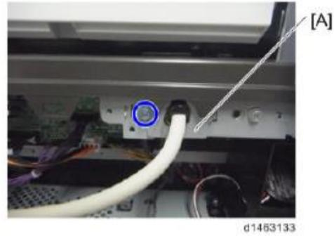
10. Remove the ADF (screws x 2)
