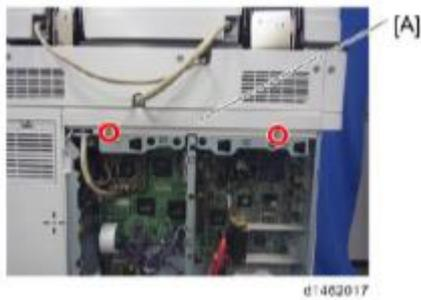
8. Remove the I/F cable [A] (screws x 2, harnesses x 1, clamps x 1)
