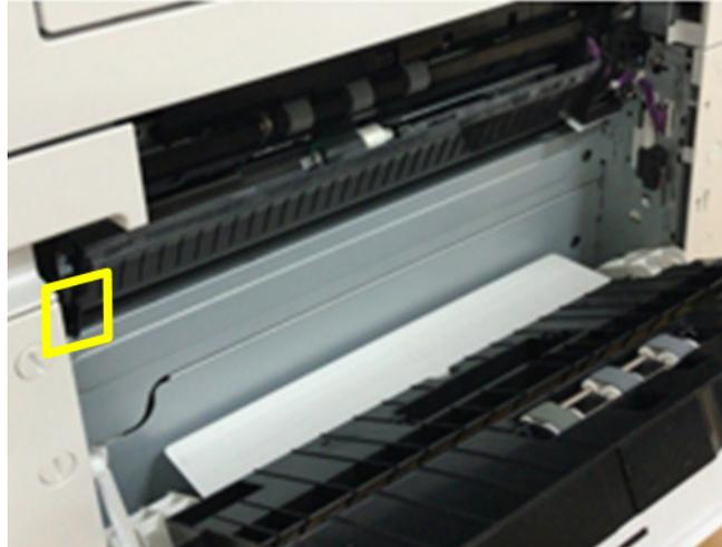
2. Attach the guide plate by sliding it toward the right hole.
