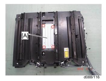
2. Polygon mirror motor cover [A] of the laser optics housing unit ( 🌶 x 4)
