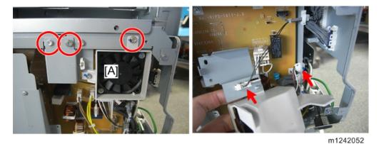
2. Duct fan with the bracket [A] ( 🌶 x 3, 📬 x 2).
