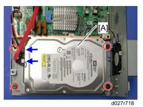
2. Remove the HDD [A] with the bracket ( x 4, 💷 x 2).
