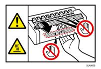
Do not touch the parts a label indicates. The inside of the machine could be very hot. Caution should be taken when removing misfed paper.
