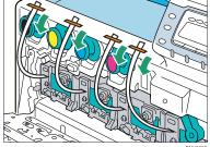
**11** Pull out the tapes horizontally. Be sure to pull out all four strips of tape.
