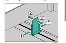
Confirm that there are no gaps between the paper and paper guides. If there are gaps, adjust the guides.
