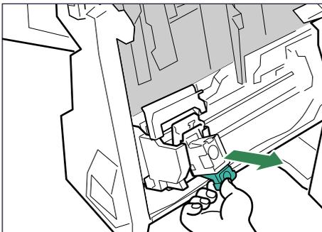
4. Pushing both sides of the cartridge, pull out the upper unit.
