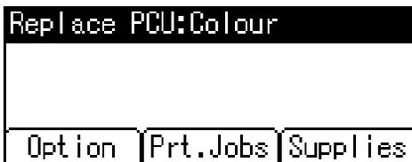
When the following messages appear on the display, the black drum unit/color drum units should be replaced soon. Prepare a new Black Drum Unit/Color Drum Unit.
