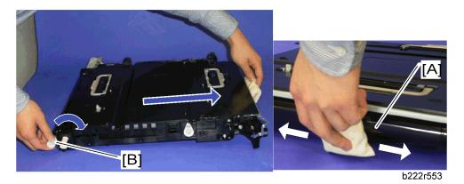
• Put "Lubricant Powder" (B132 9700) on the surface of the image transfer belt [A], while you turn the drive gear [B] at a constant speed, as shown. (The straight arrow in the picture shows belt movement direction.) Lubricant powder prevents the image transfer cleaning blade from turning up.
