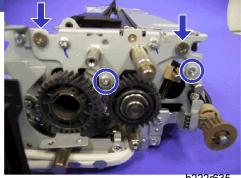
9. Upper frame [G] ( $\mathscr{F}$  x 5, stepped screw x 3, stud screw x 1)
