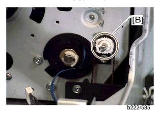
6. Remove the pulley and bushing [B].
