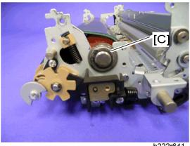
6. Fusing roller bushing [C] (C-ring x 1) at the front side
