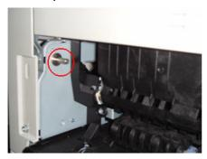
2. If the horizontal line on the printout slopes **down to the right**, attach the spring to the **non-operator side** pin.
