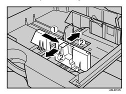
4. Pinch the clips on the end guide (1), and match the guide to the paper size (2).
