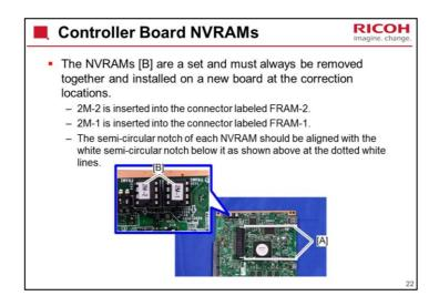
Failure to install the NVRAMs at the correct locations will cause the machine to issue SC195-00.
