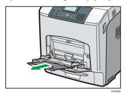
3. Slide the side guides outward, and then load paper print side down, until it stops.
