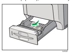
2. Push in the paper tray. Make sure the tray is securely inserted to avoid paper jams.
