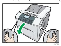
2. Tilt the duplex unit backward by carefully raising its front end.
