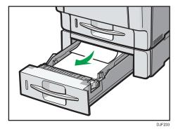
2. Carefully slide the tray back into the optional paper feed until it stops.
