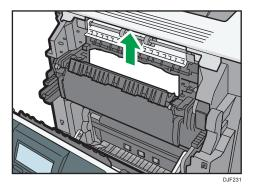
5. Close the output cover of the fusing unit.
