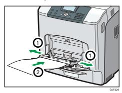
4. Adjust the side guides to fit the paper width.
