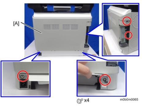
**2.** Remove the controller box cover [A].
