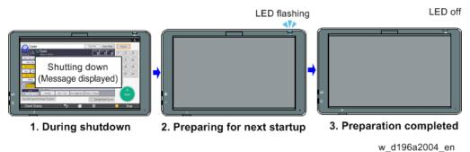
If the MFP is turned ON during shutdown, the preparation for the next startup continues. When preparation for the next startup is completed, the control panel starts up in Quick mode.
