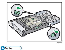
• When loading A4D,  $8^{1}/_{2} \times 11D$ , or smaller paper, do not extend the tray. Otherwise, a paper jam may occur.
