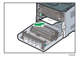
3. If the paper is jammed in the upper side of the fusing unit, pull it upward.
