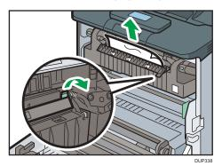
5. If you can see the jammed paper in the standard tray, keep the front cover opened and remove the paper.
