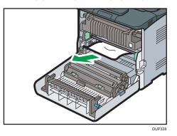
3. If you cannot see the jammed paper inside the printer, close the front cover to the position just before it is locked as shown in the illustration below.
