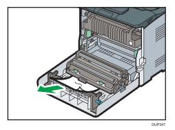
4. If paper is jammed in the upper side of the transfer unit, pull it upward.
