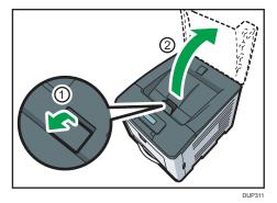
3. Pull the inner cover open lever to unlock the inner cover, and then fully open the inner cover.
