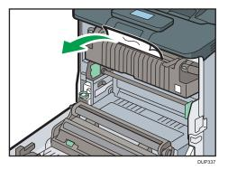
4. If you cannot see the jammed paper, pull the tabs on the fusing unit to open the cover, and then check if the paper is jammed.
