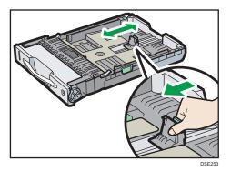
5. When loading paper into tray 1, slide the two switches at the bottom of the tray according to the thickness of the paper.
