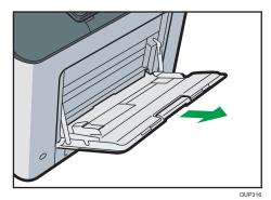
2. Slide both sides of the paper guide outward, and then load paper print side down until it stops.
