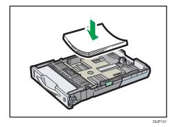
6. Set the paper straight down on the paper source tray with its printing side facing up.
