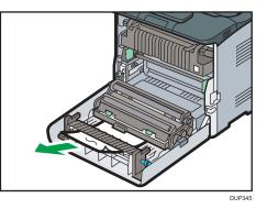
3. If you cannot pull out the paper, remove it by turning the knob on the right end of the paper transfer unit as shown in the illustration below:
