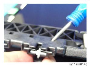
**<u>4.</u>** Remove the paper guide holder [A] and spur [B] from the image transfer belt cleaning unit [C].
