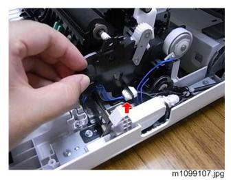
**4.** Remove the gear [A] and clip.
