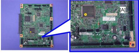
2. Install the old EEPROM on the new EGB with the mark [A] pointing as shown below.
