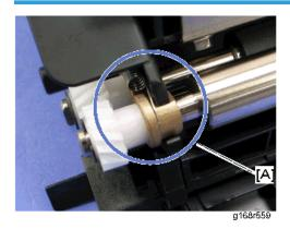
When installing the tension spring, make sure that the tension spring correctly hooks onto the bushing of the registration idle roller as shown above [A].
