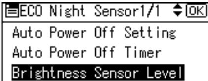
You can set the light sensor to one of five sensitivity thresholds. "Level 5 (Dim)" is the highest sensitivity threshold. Selecting this level will cause the sensor to trigger at the smallest decrease in ambient light. Selecting a lower level will cause the sensor to trigger at progressively lower levels of ambient light.
