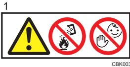
Do not incinerate spilled toner or used toner. Toner dust is flammable and might ignite when exposed to an open flame.
