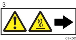
The inside of this printer becomes very hot. Do not touch parts with this label (indicating a hot surface).
