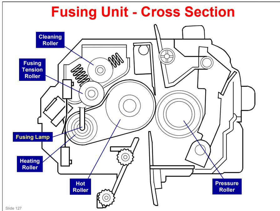
**This design, utilizing a belt between the Heating Roller and the Hot Roller, enables quick heating with the Fusing Lamp in the aluminum Heating roller, and a wider nip with the sponge Hot Roller.**
