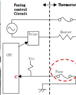
□ Thermo fuse in the new fusing unit opens when the fusing temperature reaches 72 degrees centigrade.
