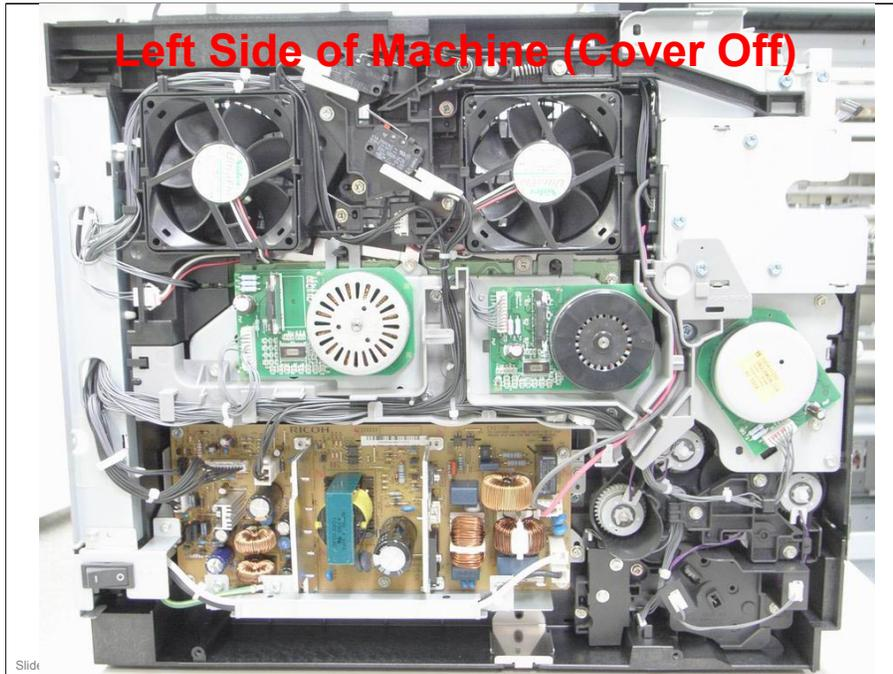
**Note that there is one less motor than the previous machine. The same functionality is achieved via a solenoid and gearing.**
