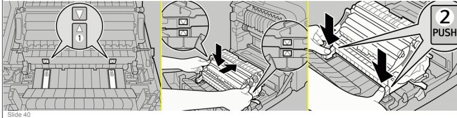
**Removing and Opening the Transfer Unit**
