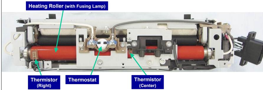
❑ View of Fusing Unit with covers removed.
