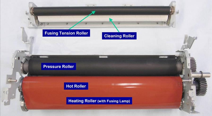
□ The five rollers within the Fusing Unit.
