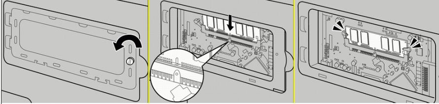
The machine has one memory expansion slot, accessed from the rear of the machine, as shown above (illustration) and below (photo).
