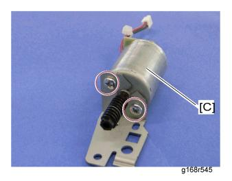
4. ITB contact motor [C] (screw x 2)
