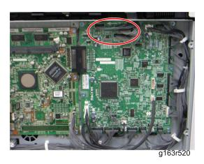
3. Disconnect the three harnesses from CN301, 302 and 303 on the EGB (connector x 3).
