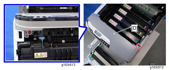
4. Operation panel [D] (screw x 2, connector x 1)
