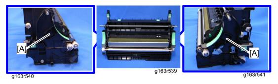
2. Release the two hooks [A] at both sides of the transfer unit.
