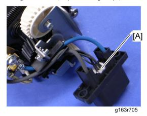
3. Disconnect the thermistor connector [A].
