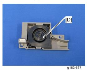
8. Air intake fan [D] (connector x 1)
