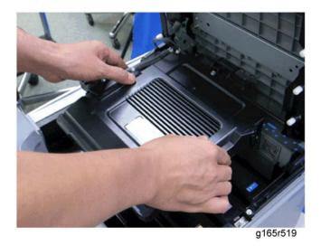
11. Remove the laser optics housing unit.
