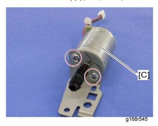
4. ITB contact motor [C] ( F x 2)
