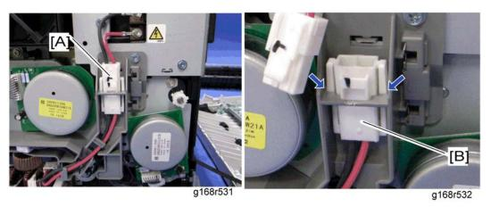
2. Disconnect the fusing connector [A] and remove the fusing relay harness [B] (hooks).
