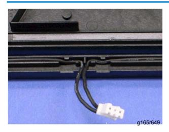
Wire the lamp cords as shown above. Otherwise, the top cover pinches the lamp cords and damages them when reinstalling the top cover on the scanner carriage unit.
