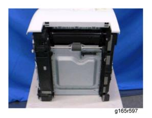
8. Stand the machine with the rear side facing the table.
