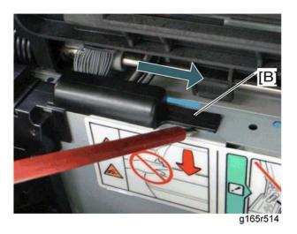
$6. \ \, \text{Lift up the hook [B] of the harness guide at the rear-left frame and slide the harness guide to the right.}$
