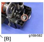
3. Fusing lamp [B] (  $\mbox{\ensuremath{\beta}}\mbox{ x 2, ground cable x 1)}$
