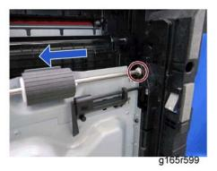
9. Slide the paper feed shaft [A] to the left side ( $\langle\!\langle\rangle\!\rangle$  x 2).
