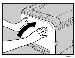
**8** Pull up Top Cover Open Lever to open the top cover.
