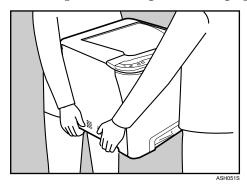
There are three upright pins on the optional paper feed unit. Align them with the holes on the underside of the printer, and then carefully lower the printer.
