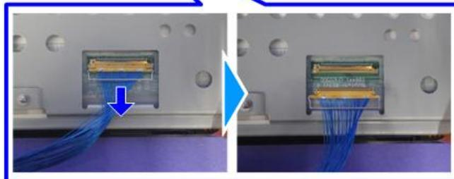
6. Remove the tapes for fixing the microphone harness (tape ×3).
