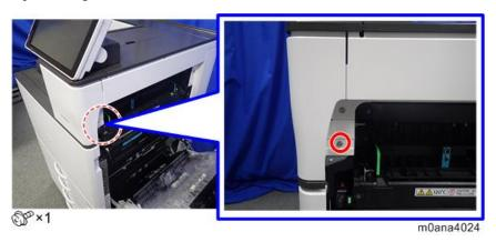
3. Release the hooks on the inside of the upper front cover [A] by pulling the cover's sides outward, and remove the upper front cover [A].
