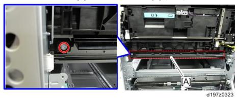
3. Release the tab on the paper dust collection unit [A]  $(\nabla \times 1)$ .
