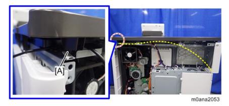
10. Clamp the cable at four points on the right side.
