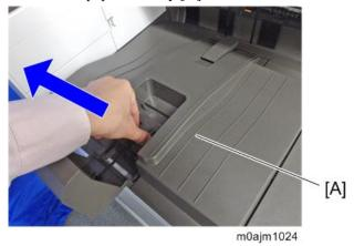
10. Open the front cover, and remove the left upper cover [A] by sliding it in the direction of the arrow.
