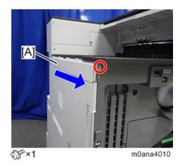
$\underline{\textbf{11.}}$  Release the hooks [A], and remove the left rear cover [B].
