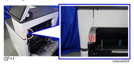
5. Release the hooks on the inside of the upper front cover [A] by pulling the cover's sides outward, and remove
