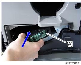
$\underline{\mathbf{3.}}$  Connect three harnesses to the new laser unit ( $\mathbf{5}^{\prime\prime}$  x 3).
