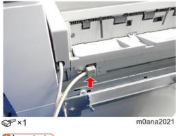
Make sure that the finisher's 2 cables are not crossing each other before you connect the finisher.
