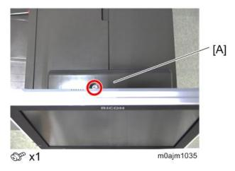
**2.** Remove the screws and clamps that secure the operation panel.
