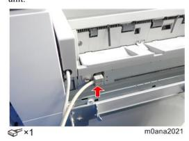
12. Remove the screw on the connection lever [A] and pull the lever.
