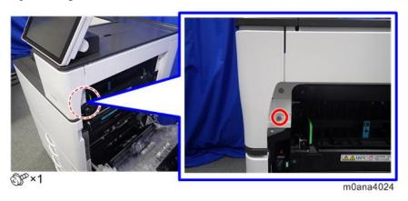
3. Release the hooks on the inside of the upper front cover [A] by pulling the cover's sides outward, and remove
