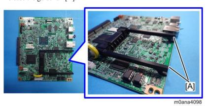
**<u>8.</u>** Remove the two used NVRAMs 1 [A] and 2 [B] from the old controller board and install them on the new
