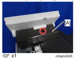
**<u>4.</u>** Remove the operation panel [A] from the machine while keeping the USB cable connected to the machine.
