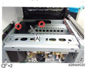
**<u>6.</u>** Remove the brackets [A] and [B].
