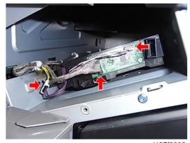
**<u>4.</u>** Insert the new laser unit along the guide frame [A].
