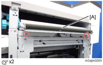
7. Attach the joint bracket [A] to the main machine (\$\mathbb{C}\text{x4: M4x12}).
