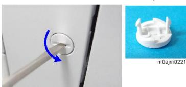
**<u>4.</u>** Attach the joint pins [A] to the front and rear on the right of the paper feed unit.
