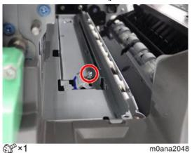
**19.** Reattach the development bearing cooling fan, PCDU, waste toner bottle, and all covers which have been removed.
