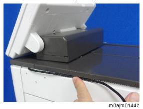
17. Attach the bracket for side table [A] to the right upper cover (M3x20).
