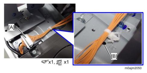
16. Insert the top right cover [A] (provided with this unit) beneath the mailbox, and secure it to the machine
