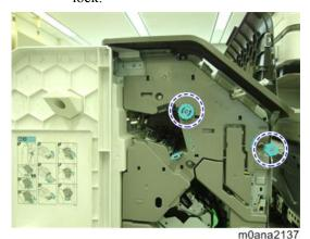
**<u>6.</u>** Remove the finisher inner cover [A] ( $\mathfrak{S}^{\times}$ 3).
