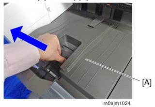
**3.** Remove the connector cover [A].
