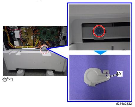
$\underline{\mathbf{5.}}$  Remove the rear cover [A] of the optional paper feed unit.
