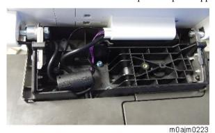
When attaching the cover, be careful not to trap the USB cable or harness between the covers.
