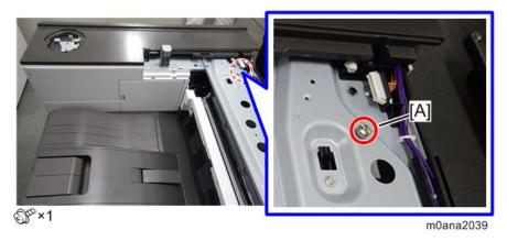
**4.** Attach the rear cover [A] provided with this unit (hook x 2).
