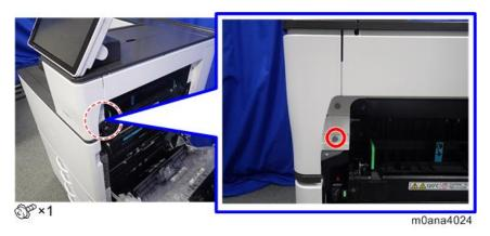
4. Release the hooks on the inside of the upper front cover [A] by pulling the cover's sides outward, and remove the upper front cover. Remove the upper front cover [A].
