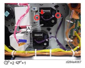
**4.** Remove the 2nd paper feed tray lift motor [A].
