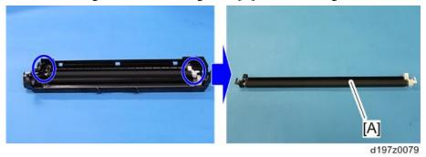
3. Split the assembly into the charge roller [A] and cleaning roller [B].
