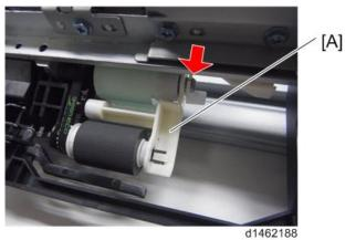
**2.** Remove the pickup roller [A].
