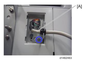
13. Attach the connector cover [A] ( $\mathfrak{O}^{\times}1$ ).
