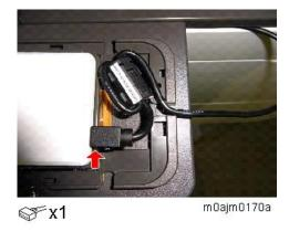
**24.** Place the NFC reader [A] on the spacer [B], and then attach the reader cover [C]. Be careful not to trap the USB cable between the covers.
