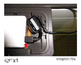
**22.** Place the NFC reader [A] on the spacer [B], and then attach the reader cover [C]. Be careful not to trap the USB cable between the covers.
