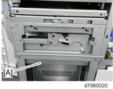
• Hook the upper frame of the hopper bracket onto the outside frame of the finisher.
