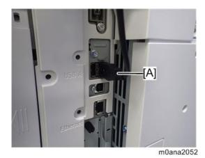
Pass the USB cable from the back to the right side of the machine.Pass the cable behind the pillar [A].
