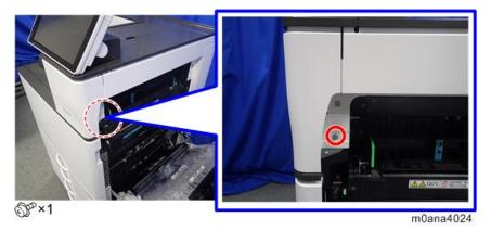
3. Release the hooks on the inside of the upper front cover [A] by pulling the cover's sides outward, and remove the upper front cover [A].
