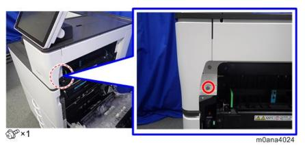
3. Release the hooks on the inside of the upper front cover [A] by pulling the cover's sides outward, and remove
