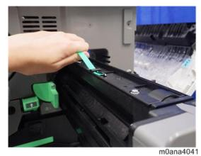
Lift the lever [A] then pull out the waste toner bottle [B].
