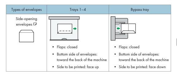
When loading envelopes, select "Envelope" as the paper types using both [Tray Paper Settings] and printer driver and specify the thickness of envelopes. For details, see "Printing on Envelopes", Operating Instructions.
