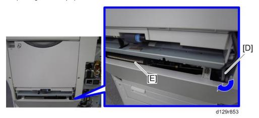
7. Push up the duplex unit a little bit, while pressing the bracket [D] to lock the spring [E].
