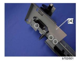
4. Remove the bracket [4] from the punch unit ( $\hat{\beta} \times 3$ ).
