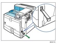
Lift the printer using the handles on both sides.
