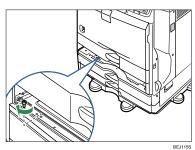
Lift the front of the tray, and slide it carefully into the printer until it stops.
