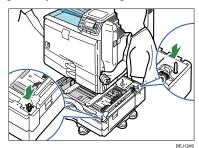
Return the handle you pulled out from the printer to its original position. Pull out tray 2 of the printer slowly until it stops, lift the front of the tray slightly, and then pull out the tray completely.
