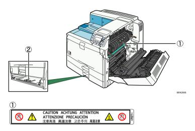
High temperature. Be careful of hot parts when clearing paper jams.
