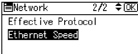
5. Press the [▼] or [▲] key to select the Ethernet speed, and then press the [OK] key.
