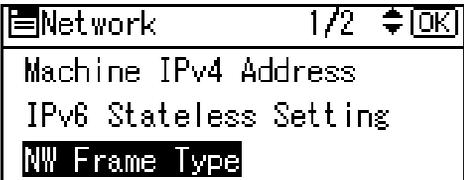
5. Press the [▼] or [▲] key to select the frame type to use, and then press the [OK] key.
