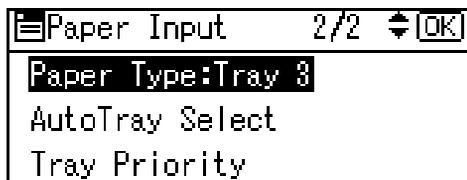
4. Press the [▼] or [▲] key to select the paper type that is loaded, and then press the [OK] key.
