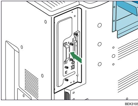
Push it firmly into the printer using the handle. The printer may malfunction if the controller board is not properly installed.
