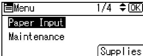
3. Press the [▼] or [▲] key to select [Paper Size: Bypass Tray,] and then press the [OK] key.
